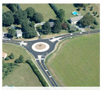
The roundabout at the intersection of Route 82 and Doe Run in East Marlborough Township is an example of a safety and circulation improvement appropriately scaled to the surrounding context.
