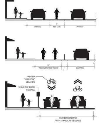
**Bike Lanes** are typically located on roadways in urban and suburban settings with moderate to high vehicular traffic volumes and moderate to high posted speeds. PennDOT's Design Manual requires a formal bike lane to be a minimum 5'width with application of pavement striping, markings, and regulatory signage. Bicycle lane facilities should be oriented for one-way operation and carry bicycle traffic in the same direction as motor vehicles
