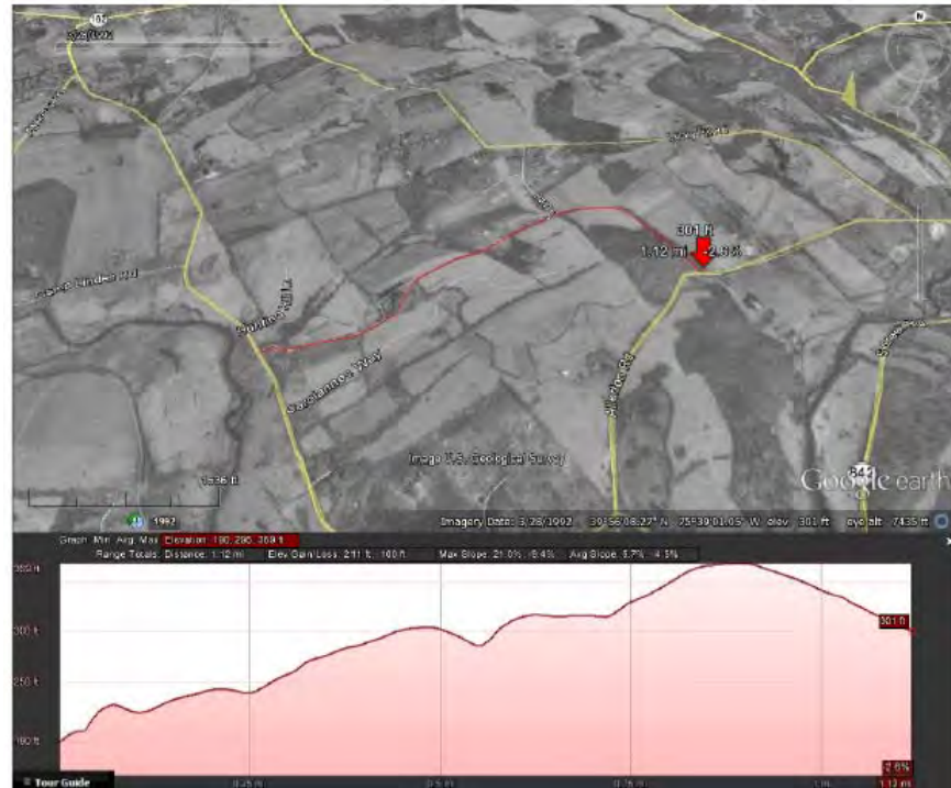
Figure 29. View of topographic profile from Google Earth of southern potential road trace.
