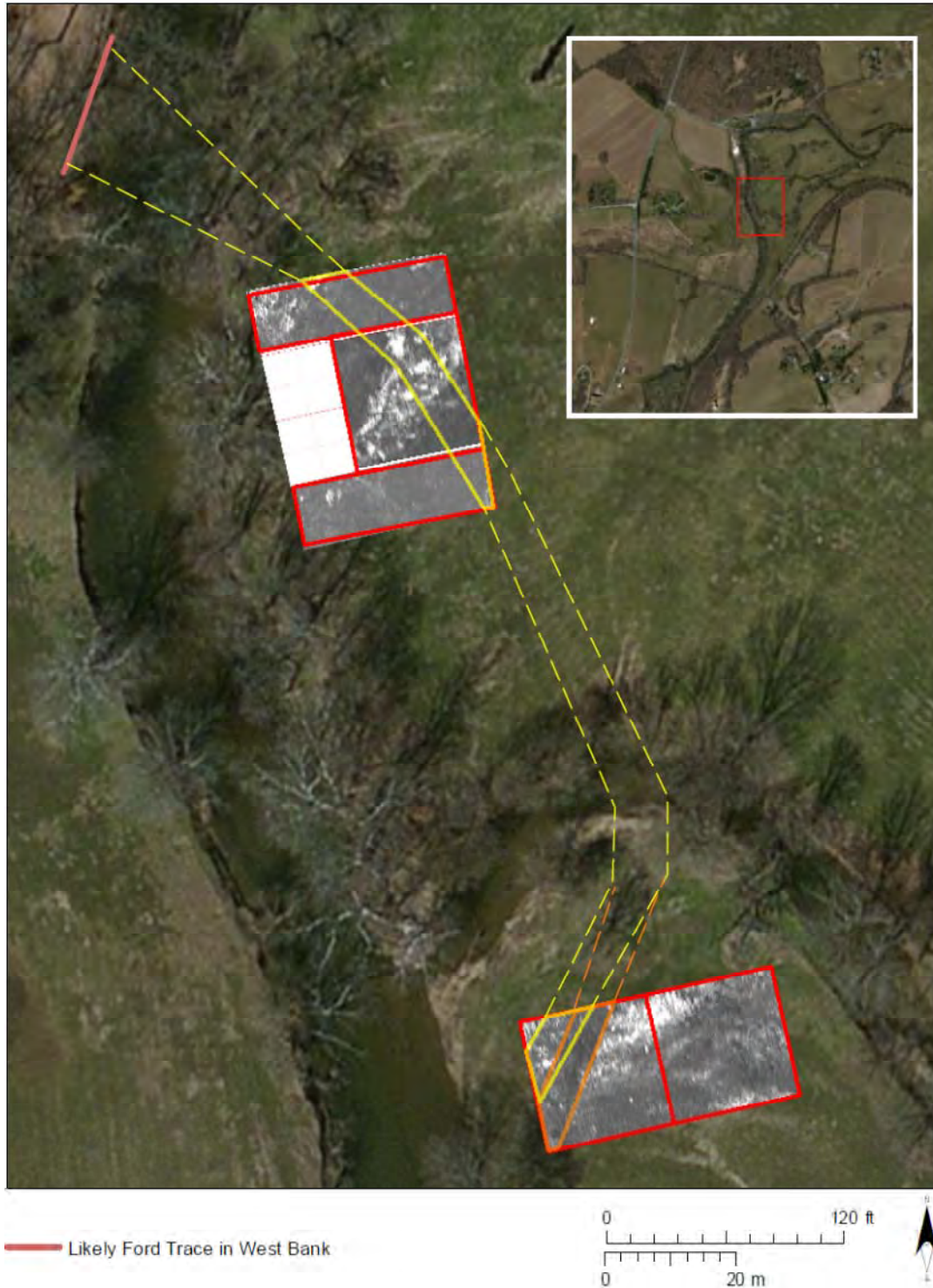
Figure 30. The locations of the potential road traces within the floodplain of the Brandywine based on the results of the geophysical survey and geomorphic testing.
